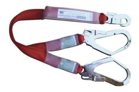
Double Shock Absorbing Lanyard with strain indicator, a standard snaphook and 2 scaffolding hooks. 1m length for use above height of 2m with fall factor of 0.
